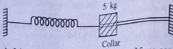
A 5 kg collar is attached to a spring of force constant  $500 \text{ Nm}^{-1}$ . It slides without friction on a horizontal rod as shown in the figure. The collar is displaced from its equilibrium position by  $10.0 \text{ cm}$  and released. The period of oscillation of the collar is -
